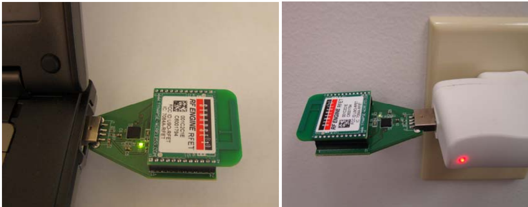
Figure 4 – A SNAPstick drawing power from a laptop PC and USB AC Adapter
