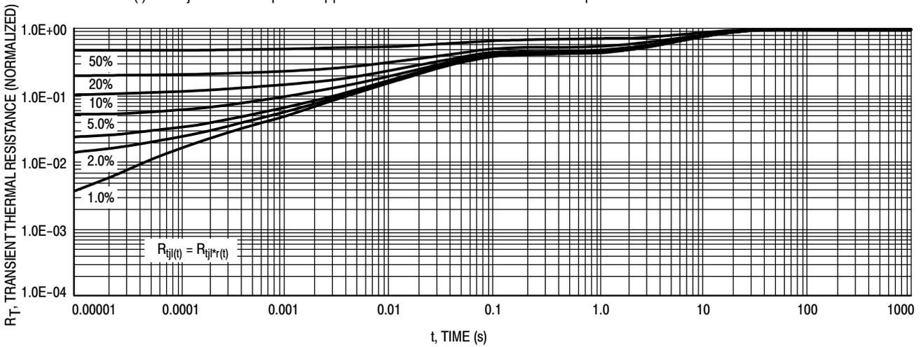
Figure 9. Thermal Response — Junction to Case
