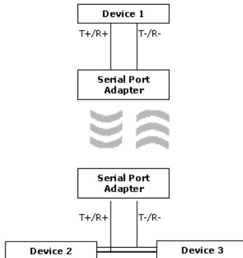
Picture 13. Two-wire RS485 connection setup
