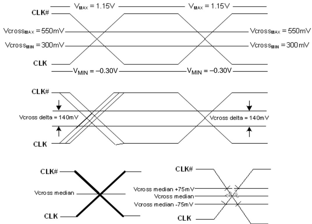
**Figure 3. Single-Ended Measurement for Differential Output Signals
