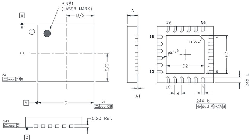
**Figure 5. 24-Pin Quad Flat No Lead (QFN) Package**
