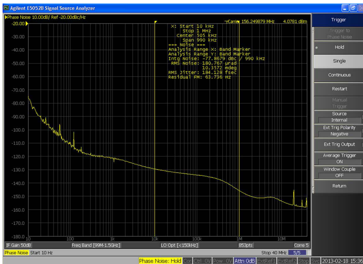
Figure 1. Si535/536 Typical Phase Noise at 156.25 MHz
