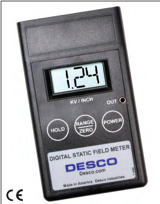
Figure 1. Desco 19492 Digital Static Field Meter
