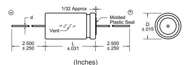
Parts are supplied with PVC insulating sleeve. Add .010" to diameter and .125" max to length to allow for insulation.
