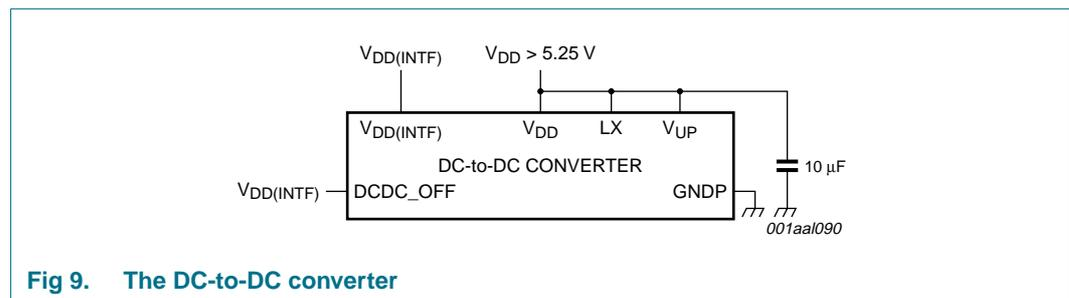
Fig 9. The DC-to-DC converter
