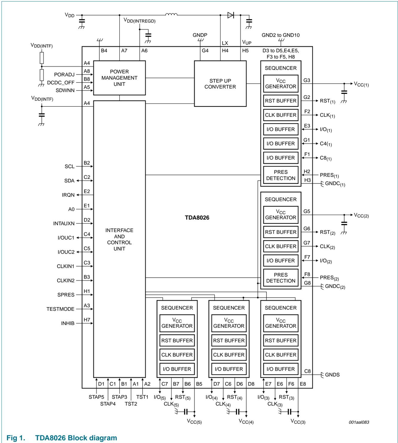
Fig 1. TDA8026 Block diagram
