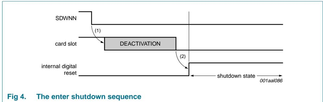
Fig 4. The enter shutdown sequence
