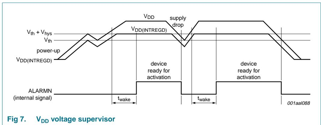
Fig 7.  $V_{DD}$  voltage supervisor
