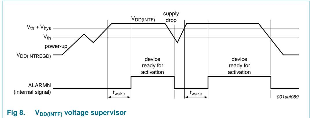
Fig 8. V<sub>DD(INTF)</sub> voltage supervisor
