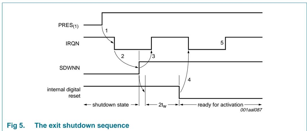
Fig 5. The exit shutdown sequence
