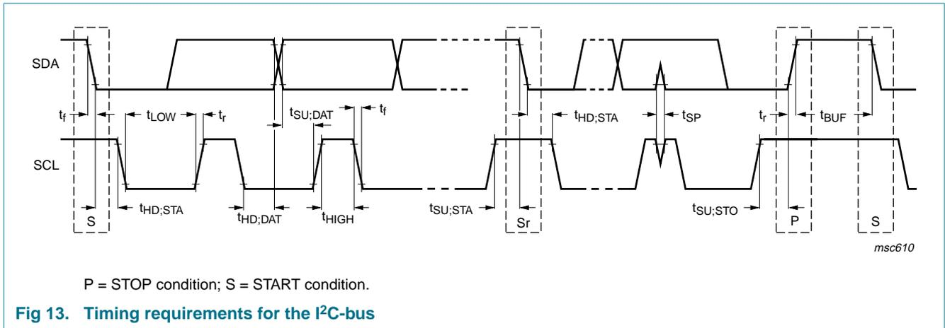
**Fig 13. Timing requirements for the I<sup>2</sup>C-bus**
