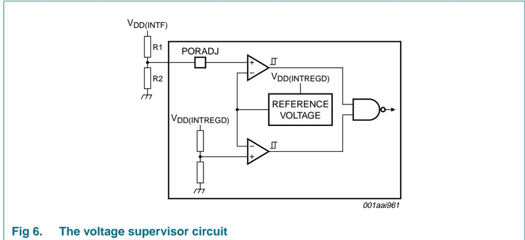
Fig 6. The voltage supervisor circuit
