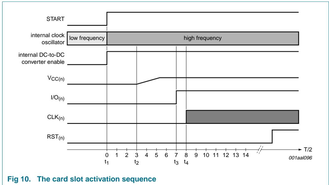
Fig 10. The card slot activation sequence
