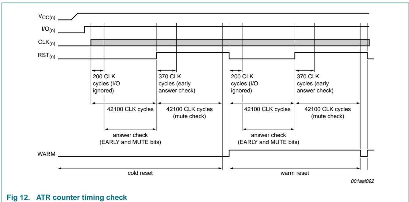
Fig 12. ATR counter timing check
