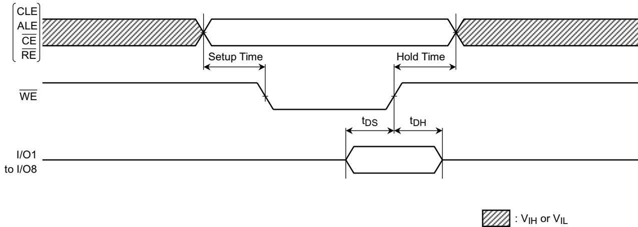
Command Input Cycle Timing Diagram
