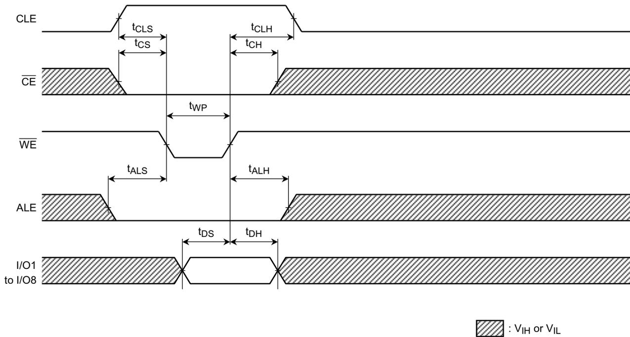
Address Input Cycle Timing Diagram
