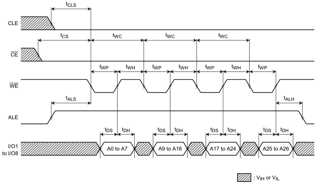
Data Input Cycle Timing Diagram
