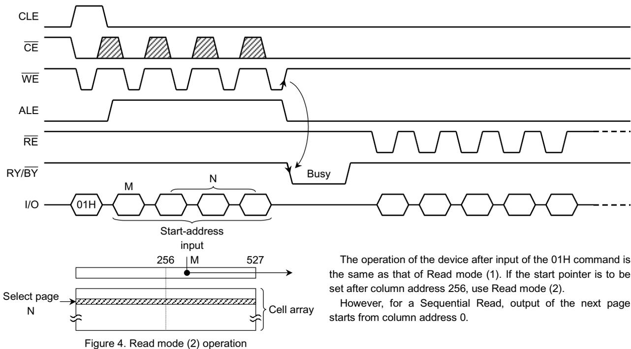
The operation of the device after input of the 01H command is the same as that of Read mode (1). If the start pointer is to be set after column address 256, use Read mode (2).
