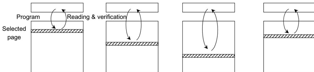
The data is transferred (programmed) from the register to the selected page on the rising edge of -WE following input of the “15H” command. After programming, the programmed data is transferred back to the register to be automatically verified by the device. If the programming does not succeed, the Program/Verify operation is repeated by the device until success is achieved or until the maximum loop number set in the device is reached.
