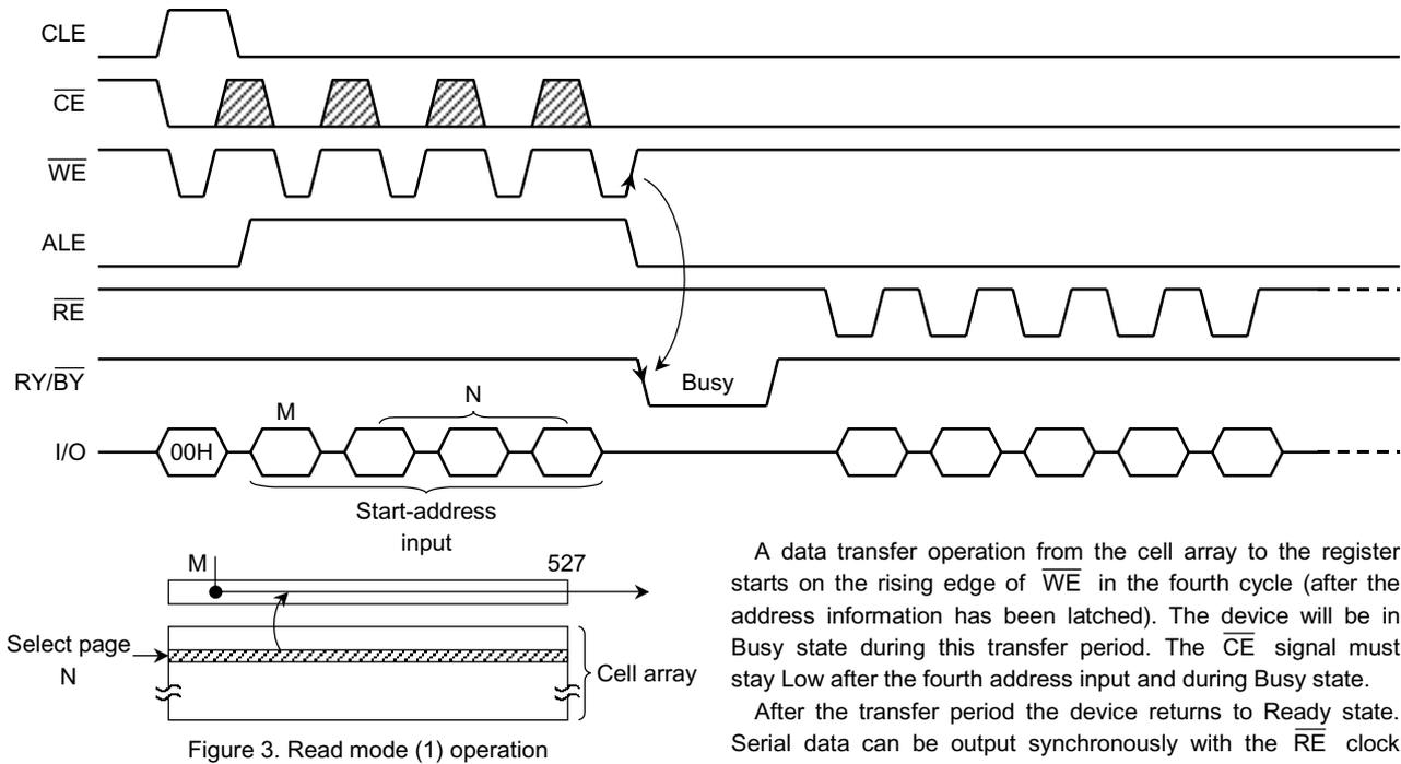
A data transfer operation from the cell array to the register starts on the rising edge of  $\overline{WE}$  in the fourth cycle (after the address information has been latched). The device will be in Busy state during this transfer period. The  $\overline{CE}$  signal must stay Low after the fourth address input and during Busy state.
