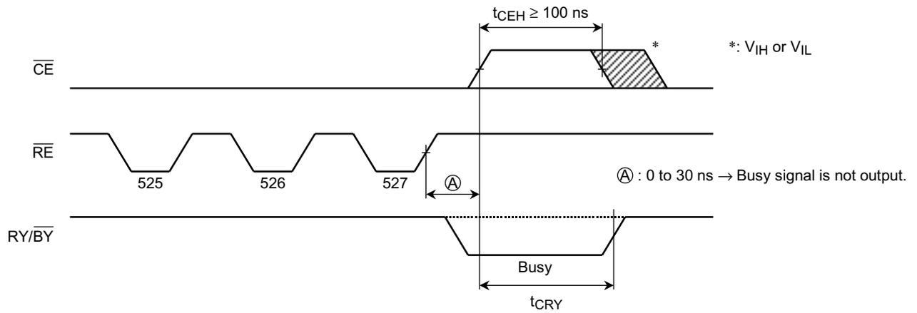
**PROGRAMMING AND ERASING CHARACTERISTICS ( $T_a = 0^\circ$  to  $55^\circ\text{C}$ ,  $V_{CC} = 3.3 \text{ V} \pm 0.3 \text{ V}$ )**
