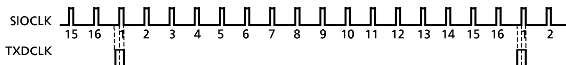
Figure 3.11 (14) Generation of Transmission Clock
