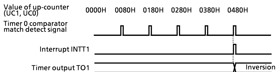
Figure 3.8 (11) Timer output by 16-bit timer mode
