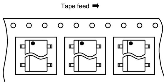
**Figure 1 Device Orientation**
