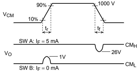
$$CM_L = \frac{800(V)}{t_r(\mu s)} \quad CM_H = \frac{800(V)}{t_f(\mu s)}$$
