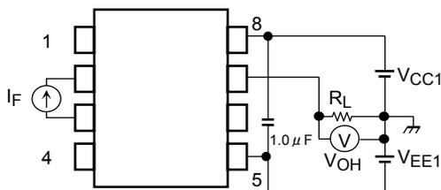
**Test Circuit 4: V<sub>OL</sub>**
