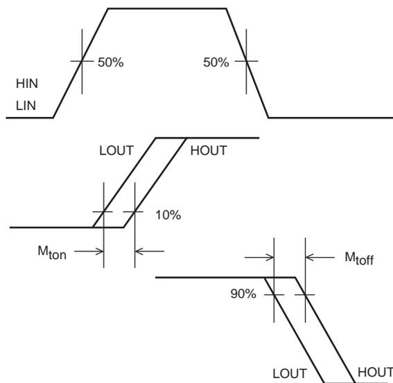
Switching Time Test Circuit
