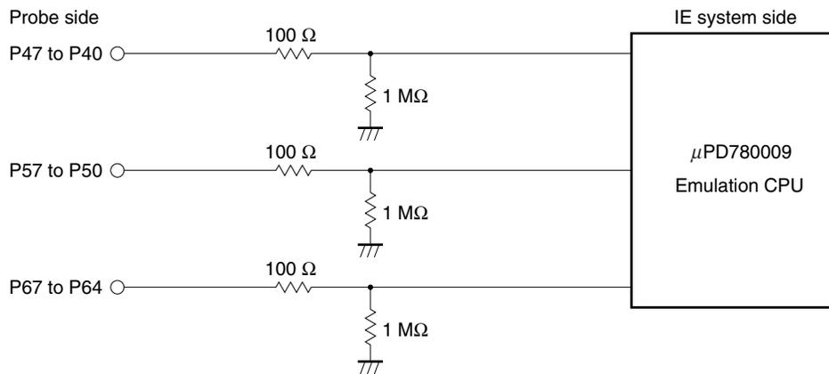
Figure 4-2. Equivalent Circuit of Emulation Circuit (2)
