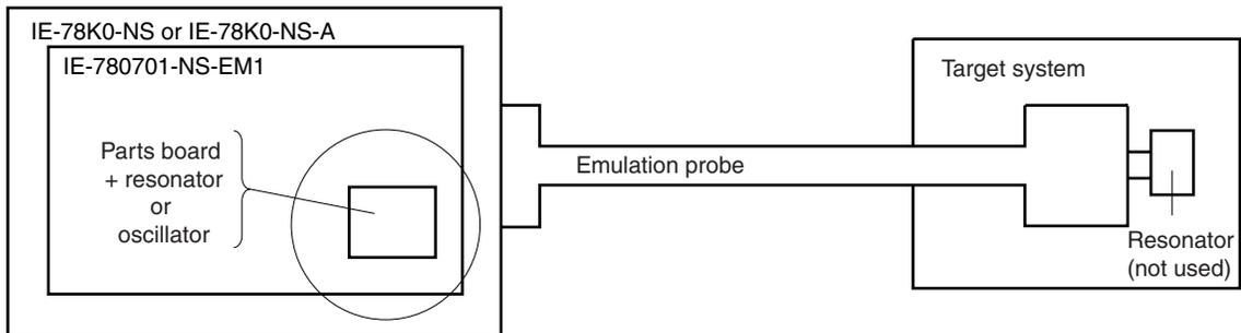
**Remark** The clock that is supplied by the IE-780701-NS-EM1's resonator or oscillator (encircled in the figure) is used.
