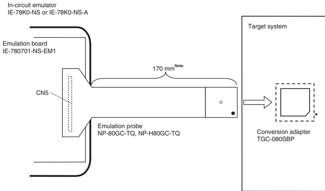
**Note** The above shows the distance when the NP-80GC-TQ is used. When the NP-H80GC-TQ is used, the distance is 370 mm.
