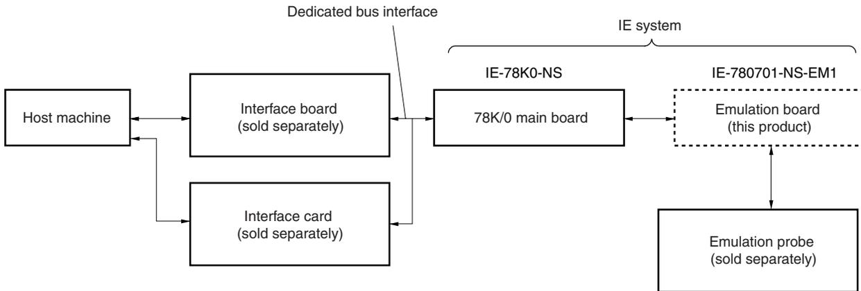
**Figure 1-3. Basic Hardware Configuration (Using IE-78K0-NS-A)**
