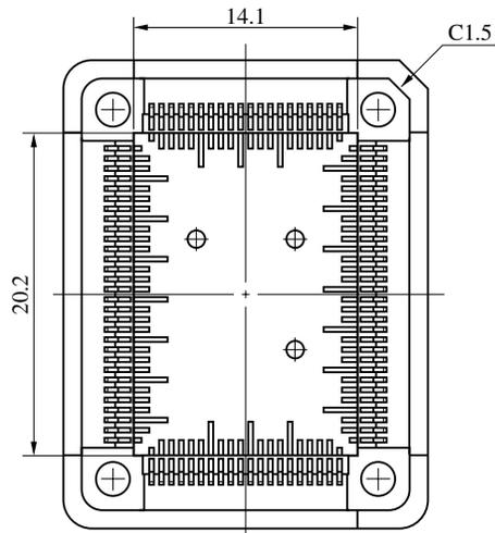
The following shows a diagram of the conditions when connecting the in-circuit emulator option board to the conversion connector. Follow the configuration below and consider the shape of parts to be mounted on the target system when designing a system.
