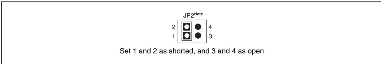
**Note** A relay is used for switching the power supply. Depending on the combinations with the target system, the relay may repeatedly turn on/off, making a continuous switching sound, when the target system is turned off. In such a case, set JP2 as shown in Figure 2-7.
