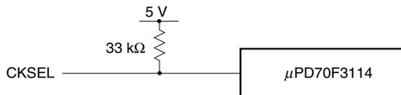
Table 5-8. Corresponding Pins (Pin Equivalent Circuit 8)
