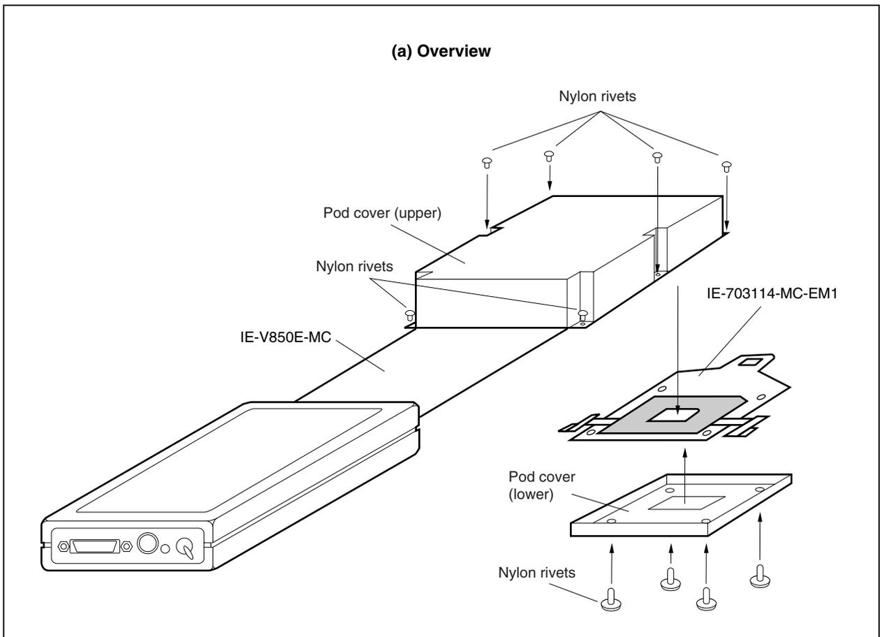
Figure 1-3. Connection Between IE-V850E-MC and IE-703114-MC-EM1 (2/2)
