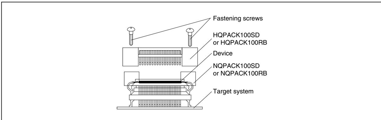
**Figure C-3. NQPACK100SD or NQPACK100RB and Device Pin**
