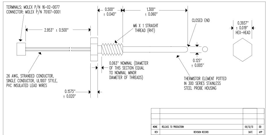
RESISTANCE @  $+25^{\circ}C = 20,000 \Omega$  NOMINAL ACCURACY ( $+50 \text{ TO } +85^{\circ}C$ ) =  $\pm 0.20^{\circ}C$  RESISTANCE/TEMPERATURE CURVE = "J" TEMPERATURE COEFFICIENT @  $+25^{\circ}C = -4.4\%$ 'C NOMINAL BETA " $\beta$ " (0 TO  $+50^{\circ}C$ ) = 3,892'K NOMINAL MAXIMUM TEMPERATURE RATING =  $+105^{\circ}C$
