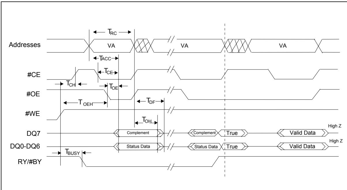
**Note:** VA= Valid Address. Illustration shows first status cycle after command sequence, last status read cycle, and array data read cycle.
