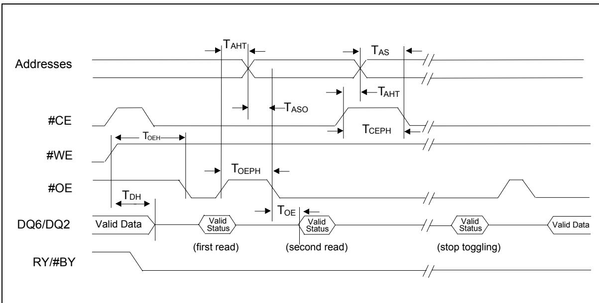
**Note:** VA= Valid address;not requires for DQ6. Illustration shows first two status cycle after command sequence, last status read cycle, and array data read cycle.
