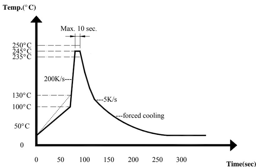
Recommendable wave soldering condition is as follows.
