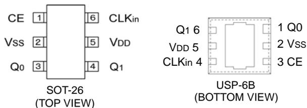
\*The dissipation pad for the USP-6B package should be solder-plated in recommended mount pattern and metal masking so as to enhance mounting strength and heat release. If the pad needs to be connected to other pins, it should be connected to the VDD pin.
