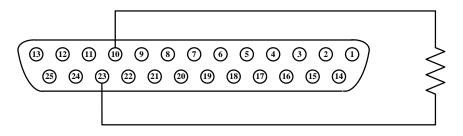
You may access MENU 6-SPECIAL TEST FUNC  $\rightarrow$  2. EXTERNAL CONTROL to choose the input resistance range at [EXTERN PROGRAM =] to [10 V / 10 K] for 0 – 10k $\Omega$  and [5 V / 5 K] for 0 – 5 k $\Omega$ .
