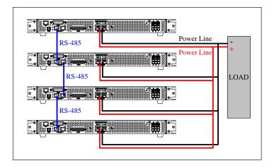
After wiring is complete, configure one of the supplies as the Master and the other three as Slave A, B, and C. After one of the supplies is configured to be the Master, it will start searching for all Slaves that are connected to the Master. To operate correctly, the user must set up the Slaves <u>before</u> the Master.
