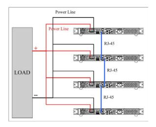
After wiring is complete, configure one XLN3640 / XLN6024 / XLN8018 / XLN10014 as the Master and the other three are Slave A, B and C. After one of the supplies is configured to be the Master, it will start searching for all Slaves
