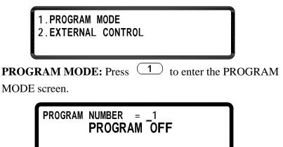
This mode allows the user to run list mode (sequences) that are stored within the internal program mode memory. Prior to using this function, the user needs to edit the list steps through the USB or GPIB interface and load it into a program memory location. Users can save up to 10 programs (program number 1 through 10) internally and recall them using this Program Mode option by selecting the program number and then pressing (On/Off) to execute the program.
