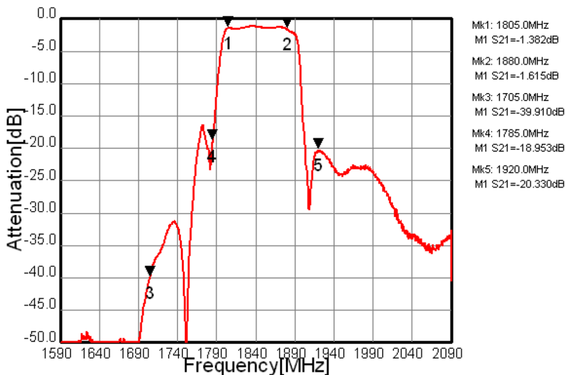
Fig.1 Pass-band Characteristic (Filter1)
