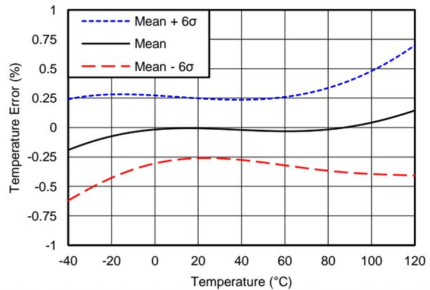
**Figure 35. INTERNAL TEMPERATURE SENSOR ACCURACY vs TEMPERATURE**
