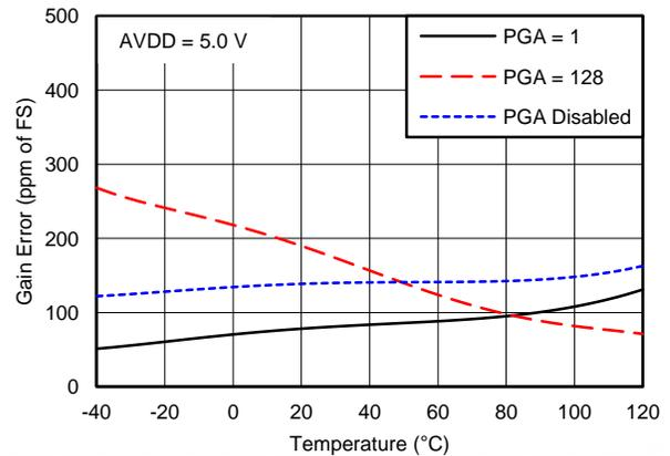
**Figure 5. GAIN ERROR vs TEMPERATURE (AVDD = 5.0 V)**
