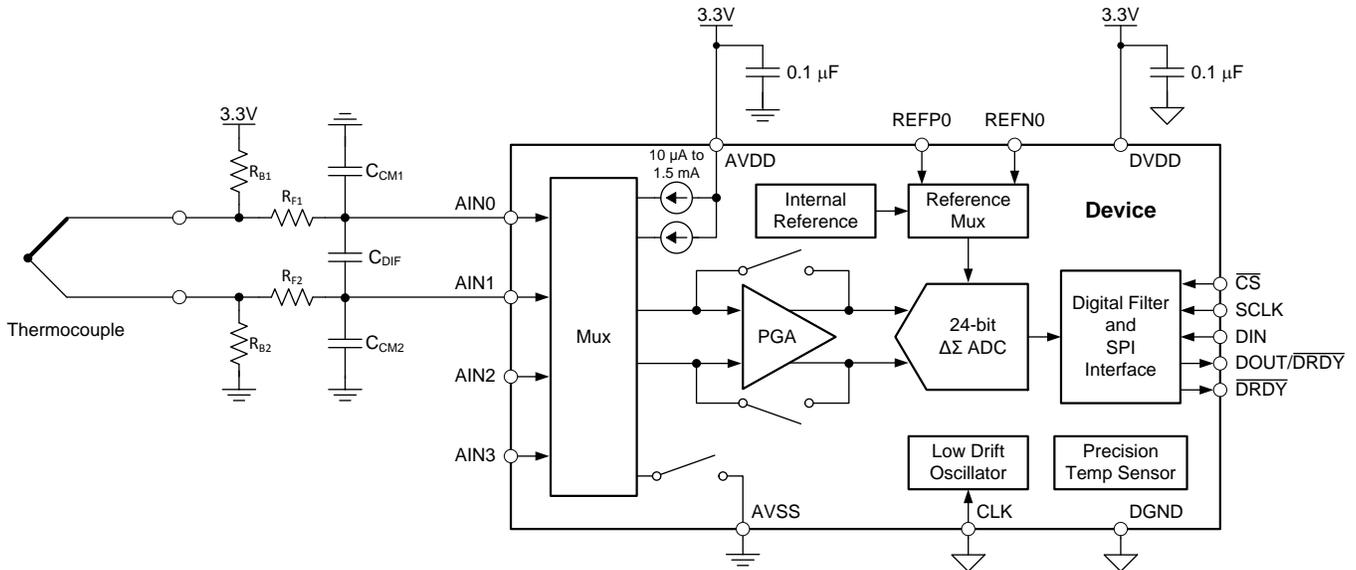
**Figure 68. Thermocouple Measurement**
