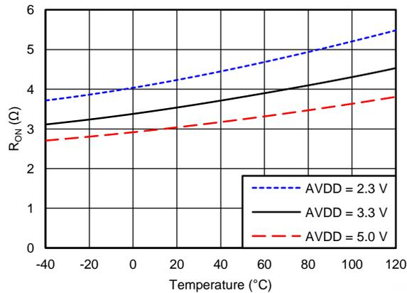
**Figure 36. LOW-SIDE POWER SWITCH  $R_{ON}$  vs TEMPERATURE**
