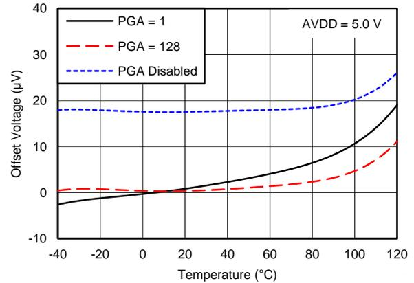
**Figure 3. INPUT-REFERRED OFFSET VOLTAGE vs TEMPERATURE (AVDD = 5.0 V)**
