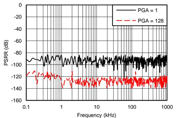
**Figure 13. AVDD POWER-SUPPLY REJECTION RATIO vs FREQUENCY**
