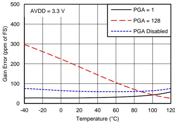
**Figure 4. GAIN ERROR vs TEMPERATURE (AVDD = 3.3 V)**
