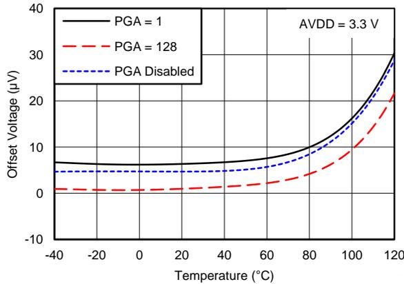
**Figure 2. INPUT-REFERRED OFFSET VOLTAGE vs TEMPERATURE (AVDD = 3.3 V)**
