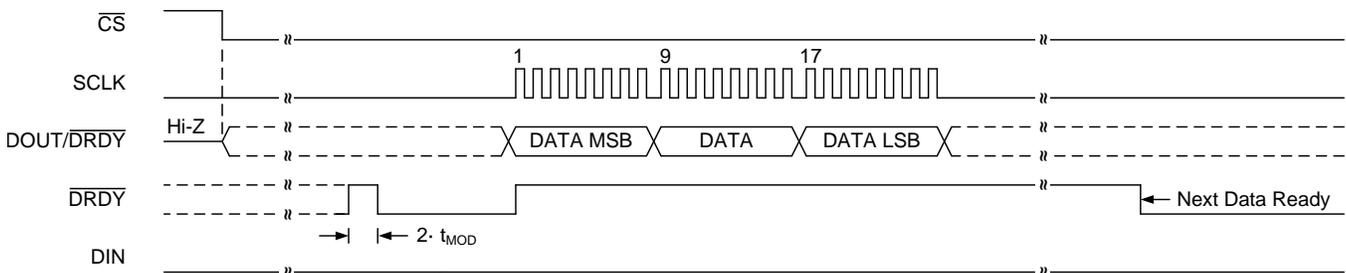
Figure 61. Continuous Conversion Mode (DRDYM = 0)
