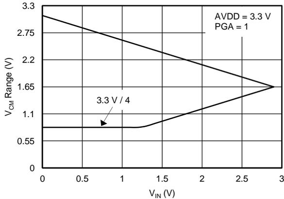
**Figure 40. Common-Mode Voltage Limits (AVDD = 3.3 V, PGA = 1)**
