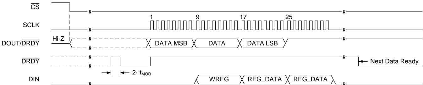
Figure 60. Example of a WREG Command
