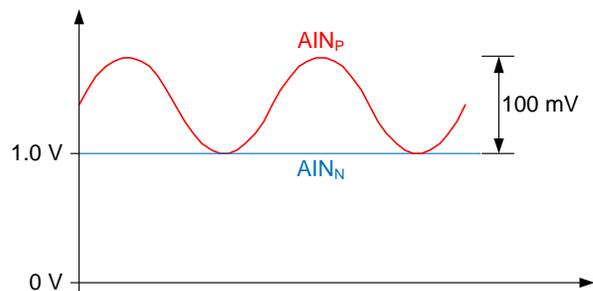
**Figure 43. Pseudo-Differential Input Signal**
