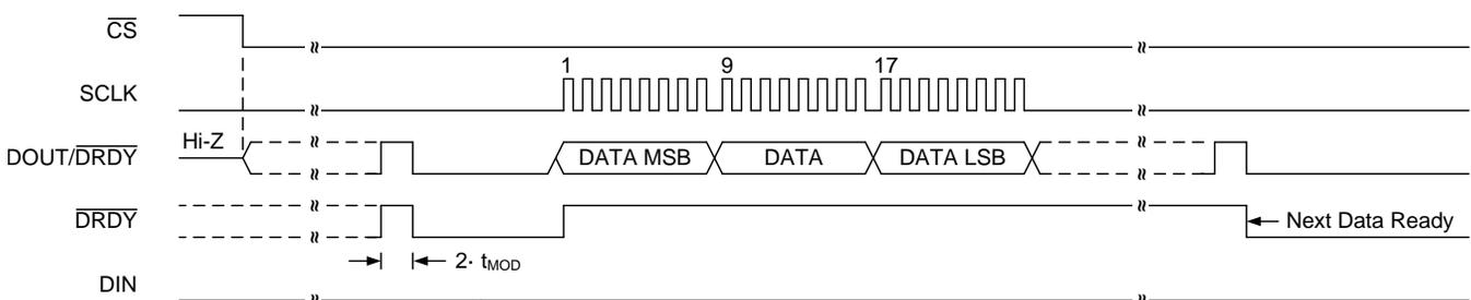
Figure 62. Continuous Conversion Mode (DRDYM = 1)
