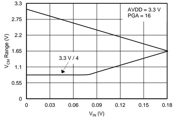
**Figure 41. Common-Mode Voltage Limits (AVDD = 3.3 V, PGA = 16)**
