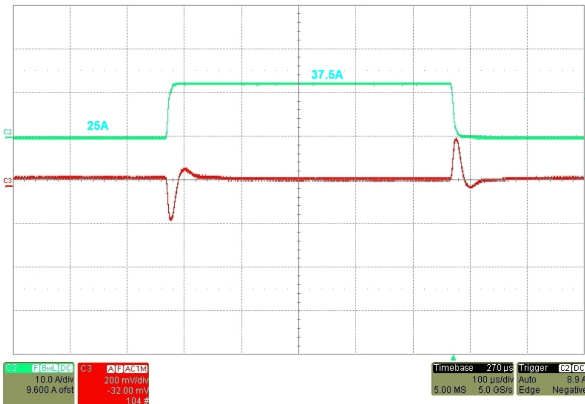
FIGURE 24. STEP LOAD: 25A TO 37.5A (12.5A DELTA)
