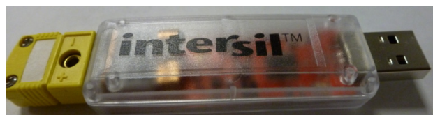
FIGURE 1. DAQ ON A STICK WITH THERMOCOUPLE
