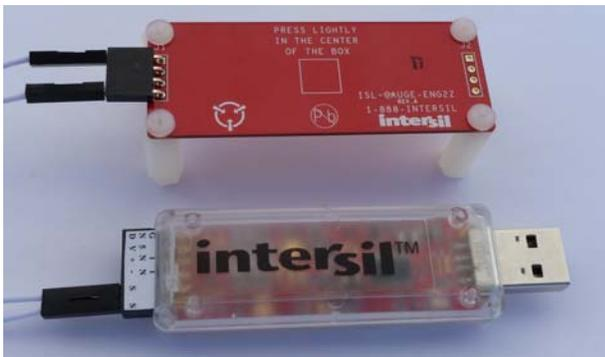
FIGURE 1. DAQ ON A STICK WITH STRAIN GAUGE
