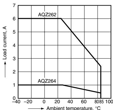
2. Load current vs. ambient temperature characteristics in adjacent mounting
