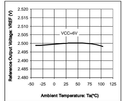
Fig.6 VREF temperature characteristics
