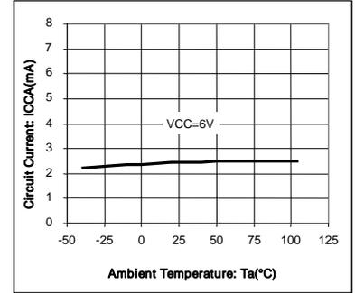
Fig.3 Circuit current temperature characteristics in operation
