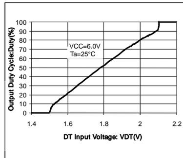
Fig.20 Output Duty-VDT characteristics (1.5MHz)
