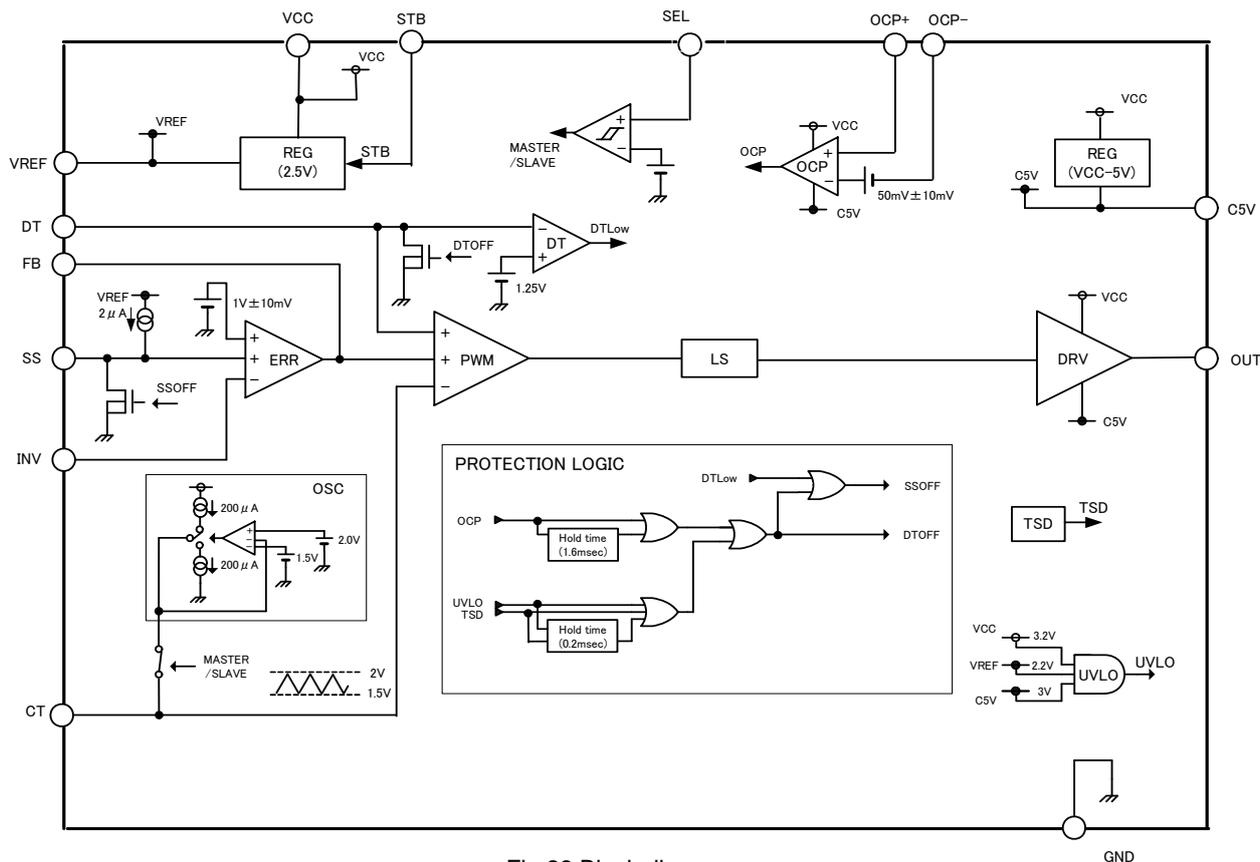
Fig.28 Block diagram
