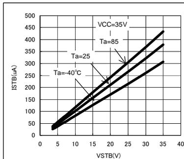
Fig.23 STB flow-in current
