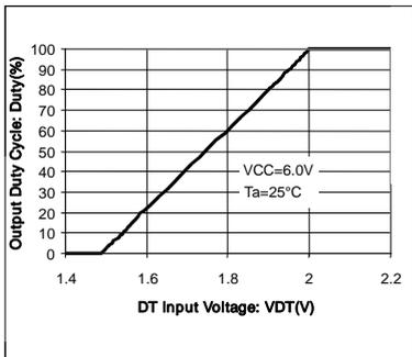
Fig.19 Output Duty-VDT characteristics (100kHz)
