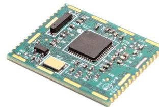
**ZigBee/802.15.4.** The ZMN2430 includes the ZigBee 2006 stack as well as Cirronet's CSM profile eliminating the need for any firmware development. The ZMN2430 can operate as a reduced function device (RFD) for end devices to consume the least amount of power, or as a full function device (FFD) to act as a Coordinator or Router. Each node type can be ordered separately or the module's bootloader can be used to load the appropriate firmware during manufacture.
