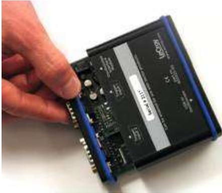
7. Slide the tray back into the housing, making sure that when the tray is re-installed the USB connector is showing.
