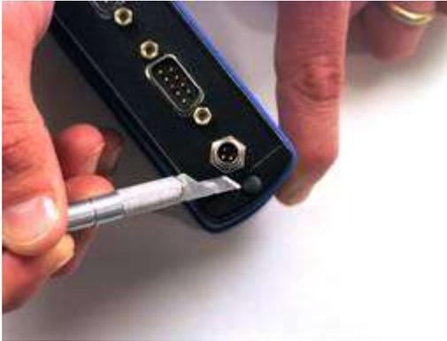
2. The housing is shipped with two of the plastic end caps (that cover the screws) uninstalled. If these have been installed by you or someone else, you will need to remove them with a small screwdriver or knife.
