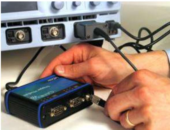
4. Connect the 3-pin plug end of the OIM to the Trigger Module.
