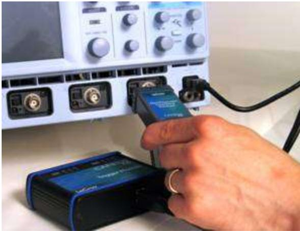
3. Connect the CANbus TD/TDM Oscilloscope Interface Module (OIM) to the EXT input of the instrument. Make sure that the top (OIM labeled side) is facing up.
