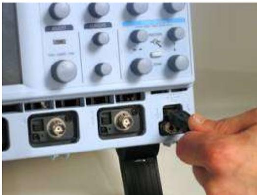
1. Connect the USB2.0 Cable to one of the instrument's PC-USB ports.
