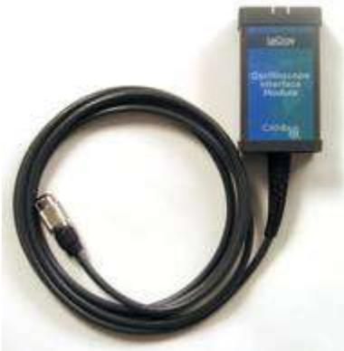
Qty. 1: **Oscilloscope Interface Module** -- This module connects to the Trigger Module via the 3-pin connector. The module is LeCroy ProBus<sup>®</sup> compatible. When plugged into a LeCroy oscilloscope, it is automatically recognized and proceeds with appropriate setup for CAN triggering. The OIM can be connected to any channel, but is more commonly connected to the EXT input (to reserve a channel for an analog signal). Once connected, it sets the following:
