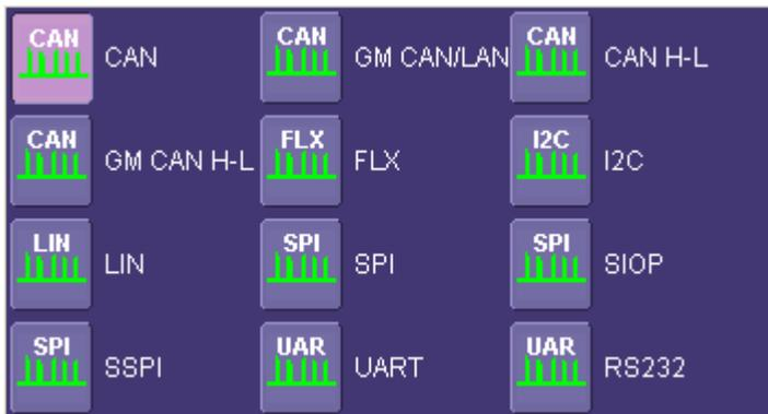
4. **Measure/Graph Setup** - CAN measurement and graphing functions are accessed through the Serial Decode setup by selecting the Measure/Graph Setup tab.
