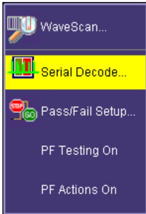
3. **Decode Protocol Selections** - As serial decode options are added to your oscilloscope, additional protocol selections are available in a pop-up dialog box within the Serial Decode dialog boxes.
