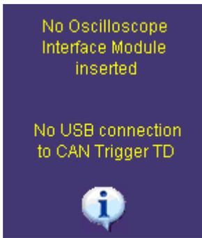
If you see either or both of these error messages (shown in the picture to the right) in the CAN Trigger dialog, then you need to re-examine the connections to the Trigger Module and make sure that they are correct. This message will be replaced by Trigger Module attributes and trigger coupler information when the Trigger Module is properly connected.
