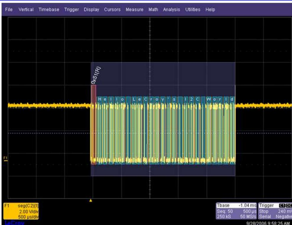
9. View the timestamps for each segment by selecting **Vertical**→**Channels Status** on the menu bar. On the **Show Status** portion of the dialog, select Time. A display of timestamp information for each segment in the sequence acquisition is shown.
