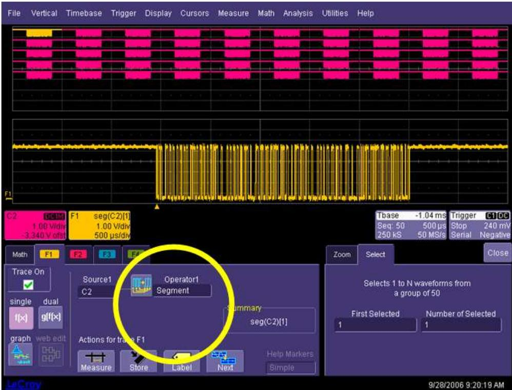
7. Set up the Decode to use the Math trace as the source for Data in order to view decoded data on the individual segment (in this case F4 is the source).
