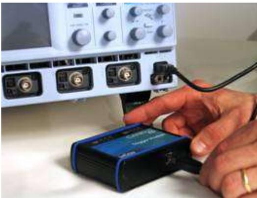
2. Connect the other end of the USB2.0 Cable to the CANbus TD/TDM Trigger Module.
