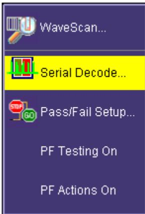
3. **Decode Protocol Selections** - CAN is one of several signal types that can be decoded by the oscilloscope. Other standards include I2C, SPI, UART, RS-232, LIN, and FlexRay.
