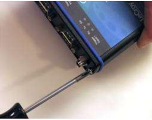
3. Unscrew the screws on the DSUB-9 connector side of the Trigger Module using a Philips #1 screwdriver.
