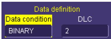
**Binary Data Condition** – The CAN trigger can be set up in binary format by selecting a “Binary” Data Condition in the Data Definition section of the CAN Trigger dialog. You might want to choose binary format setup when you want to trigger on less than full nibbles of data, or when you want to trigger on more than 24-bits of data.
