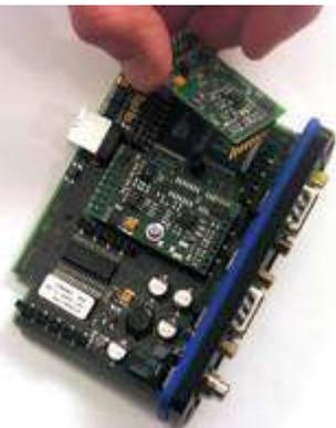
5. The Trigger Coupler is held down with a screw and locknut. Use a Philips #1 screwdriver to remove them. If necessary, carefully remove a Trigger Coupler from the main board, taking care not to touch the bottom of the Trigger Coupler. Store the Trigger Coupler in one of the static sensitive boxes (provided).
