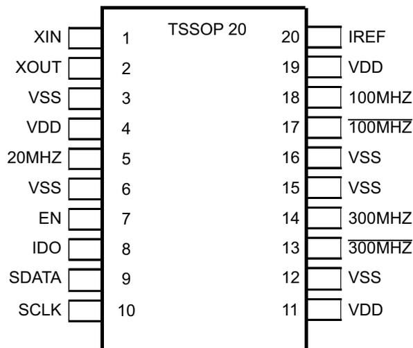
The 100 MHz HCLK output provides the reference clock for the XDR Clock Generator (CDCD5704). Spread-spectrum clocking with 0.5% down spread, which reduces Electro Magnetic Interference (EMI), is applied in the default configuration. The spread-spectrum clocking (SSC) is turned on and off via the serial control interface.
