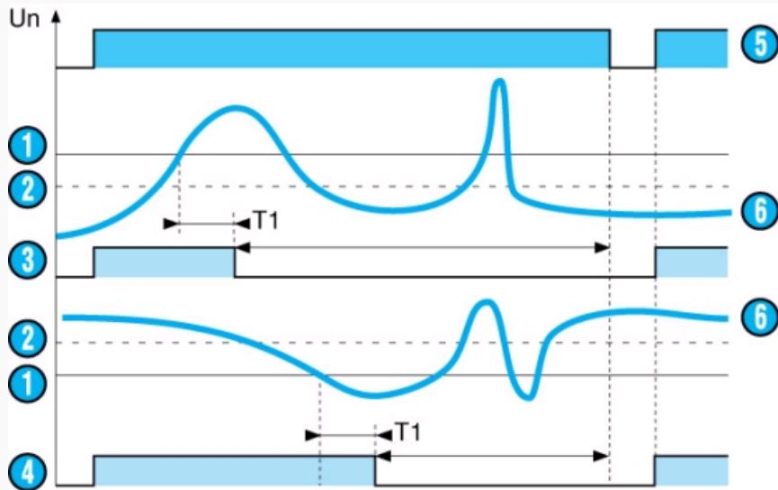
When the value of the controlled voltage, AC or DC, reaches the threshold  $U_e$  displayed on the front face, the output relay changes state at the end of a time delay  $T_1$ , which can be set on the front
