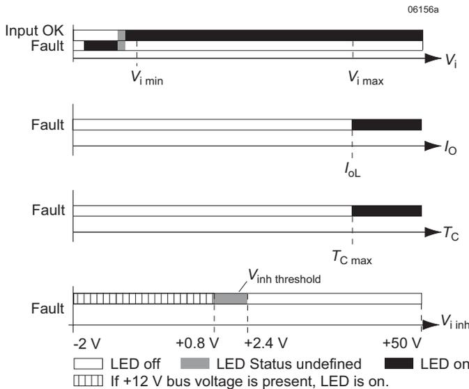
LEDs "Input OK" and "Fault" status versus input voltage.
