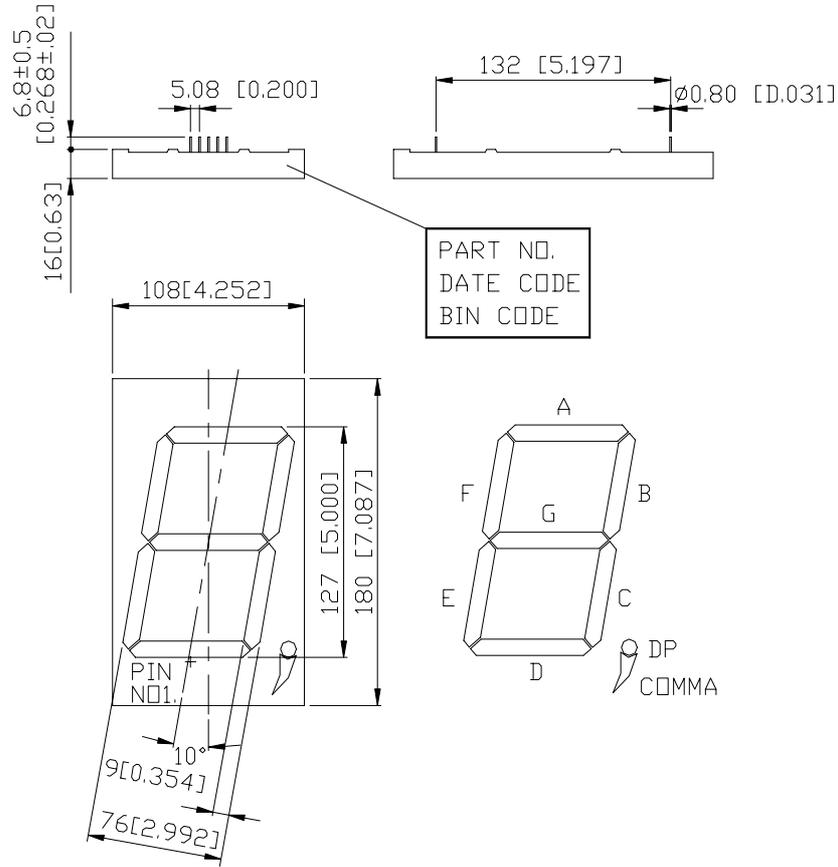
NOTES: All dimensions are in millimeters. Tolerance is  $\pm 0.25\text{mm}(0.01\text{'})$  unless otherwise noted.
