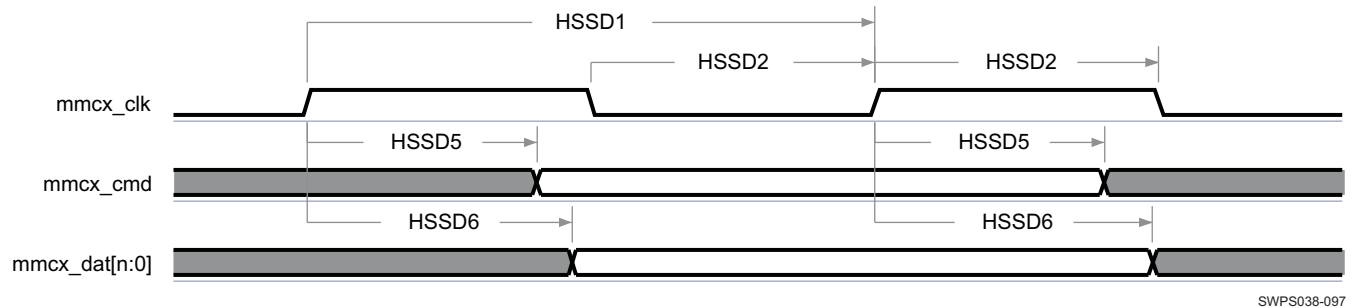
Figure 6-74. MMC2 and MMC3 Interfaces—High-Speed SDIO Mode—Data/Command Transmit (1)
