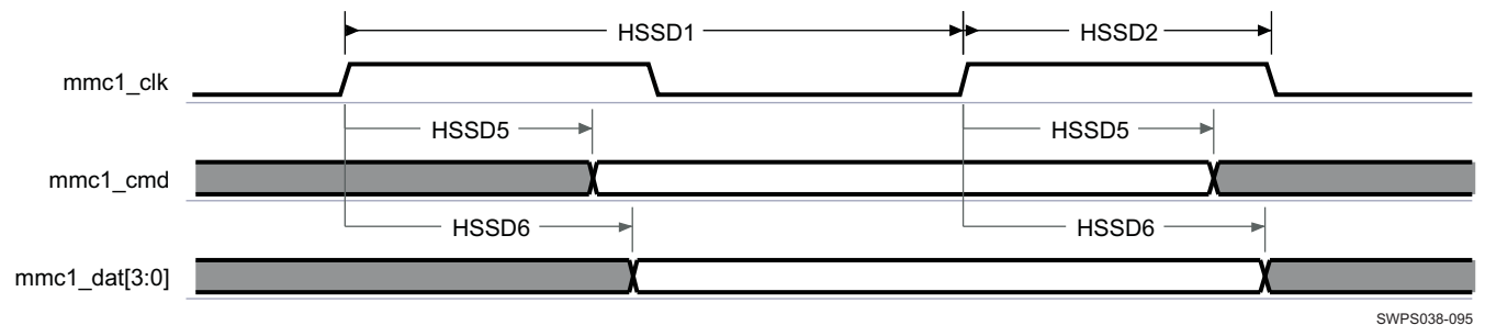
Figure 6-66. MMC1 Interface—High-Speed SD Mode—Data/Command Transmit
