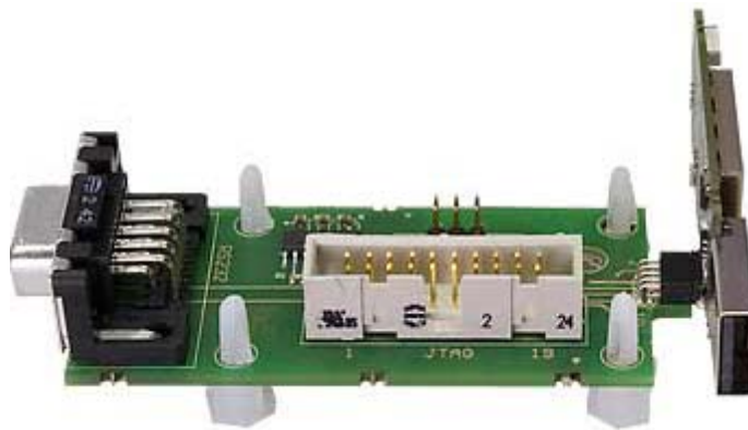
Figure 6-1. SAM-ICE adapter PCBA connected to the RF231USB PCBA.
