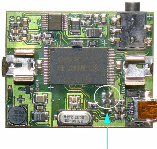
Solder two SMD 0 $\Omega$  resistors here (horizontally).
