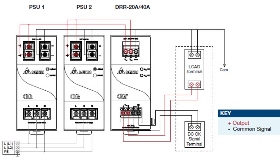
Fig. 3.1 Redundancy / Parallel Operation Connection Diagram
