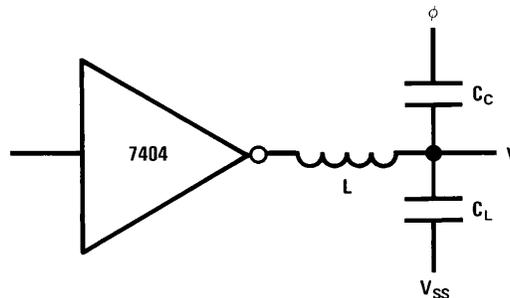
Figure 17. Clock Coupling
