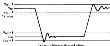
**Figure 15. Clock Waveform**
