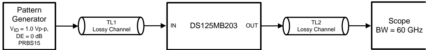
Figure 22. Test Setup Connections Diagram
