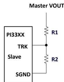
Figure 6 - Voltage divider connections for direct tracking
