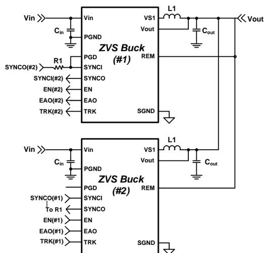
Figure 3 - PI33XX-X0 parallel operation
