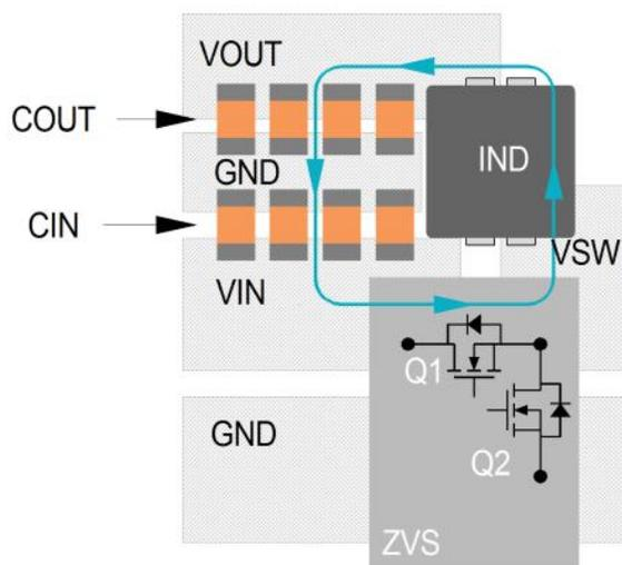
Figure 12 - Recommended component placement and metal routing
