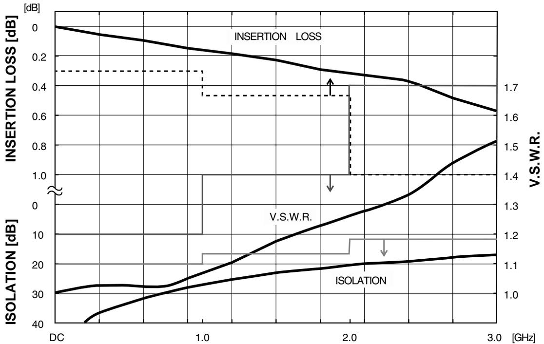
**MS-151NB Series** Interface RF Connector with Switch, built-in interlock, DC to 3GHz
