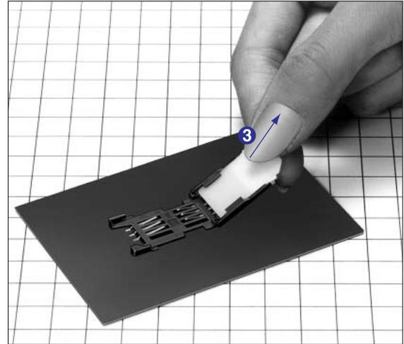
Remove the SIM card (as shown) so that it comes out from the card holder.
