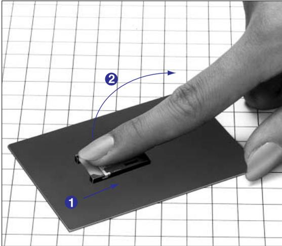
Press the slider and at the same time move it in the direction marked "OPEN". This action will release the lock and free the card holder.
