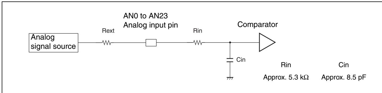
The output impedance of the external circuit connected to the analog input affects the sampling time of the A/D converter. Design the output impedance of the output circuit such that the required sampling time is less than the value of  $T_s$  calculated from the following equation.
