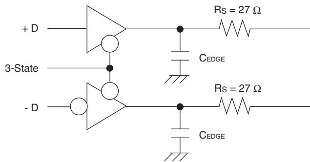
Driver output impedance 3  $\Omega$  to 19  $\Omega$
