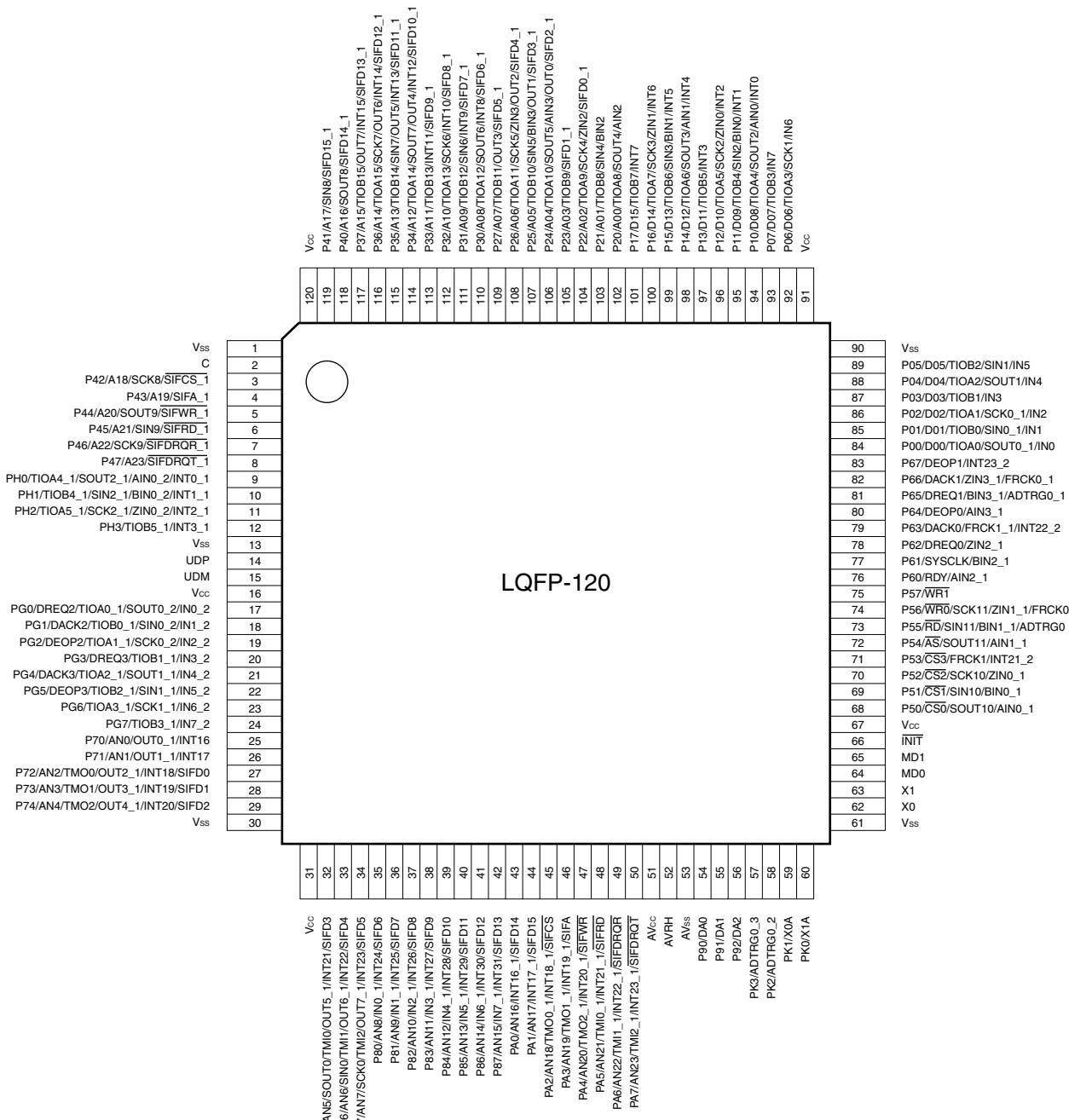
Note : The number after the underscore ("\_) in pin names such as XXX\_1 and XXX\_2 indicates the port number. For these pins, there are multiple pins that provide the same function for the same channel. Use the extended port function register (EPFR) to select the pin.
