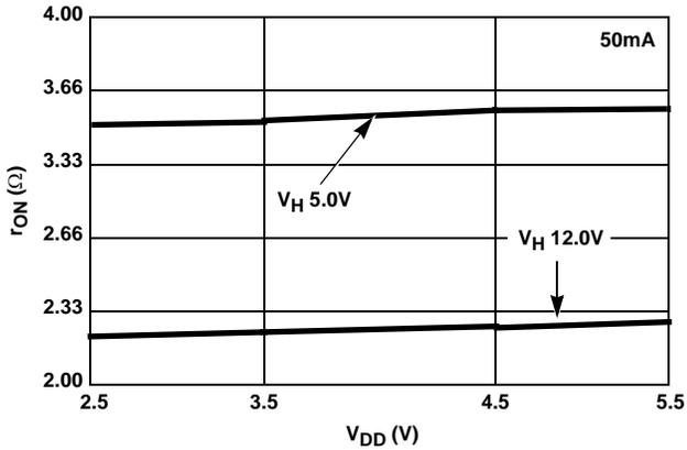
FIGURE 5.  $r_{ON}$  vs  $V_{DD}$  SOURCE RESISTANCE
