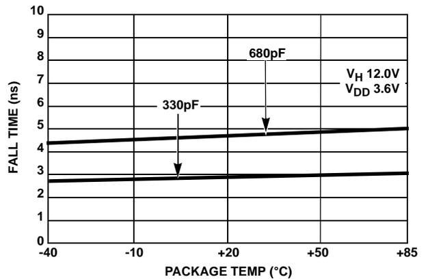
FIGURE 16.  $t_F$  vs TEMPERATURE
