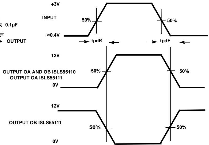
$$t_{\text{SKEW R}} = t_{\text{pdR CHN1}} - t_{\text{pdR CHN2}}$$
