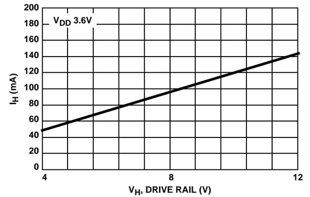
FIGURE 10.  $I_H$  vs  $V_H$  @ 50MHz (NO LOAD)
