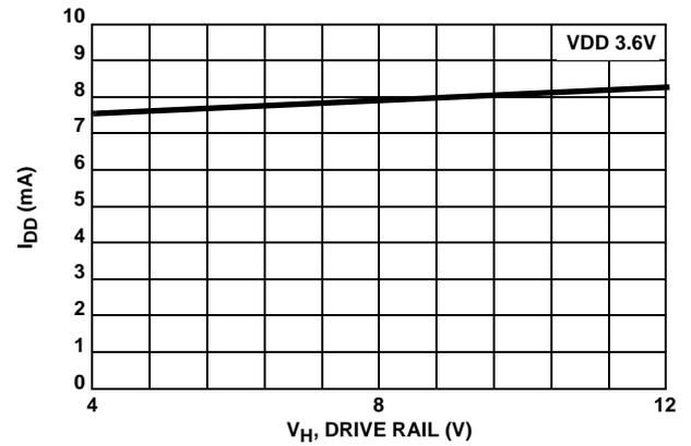
FIGURE 8.  $I_{DD}$  vs  $V_H$  @ 50MHz (NO LOAD)
