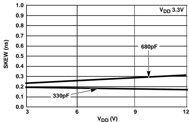
FIGURE 31. tSkewR vs V<sub>H</sub>
