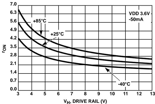
FIGURE 3. DRIVER  $r_{ON}$  vs  $V_H$  SOURCE RESISTANCE
