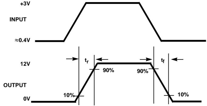
FIGURE 1. TEST CIRCUIT RISE ( $t_R$ )/FALL( $t_F$ ) THRESHOLDS
