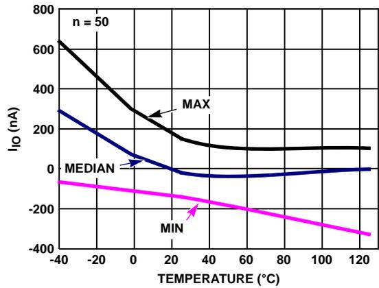
FIGURE 24.  $I_{IO}$  vs TEMPERATURE  $V_S = \pm 2.5V$
