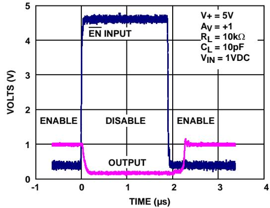
FIGURE 16. ENABLE/DISABLE TIMING
