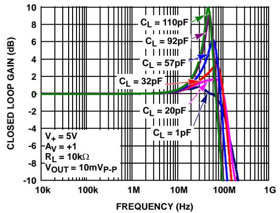
FIGURE 2. GAIN vs FREQUENCY FOR VARIOUS  $C_{LOAD}$
