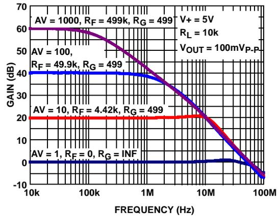
FIGURE 4. FREQUENCY RESPONSE vs CLOSED LOOP GAIN
