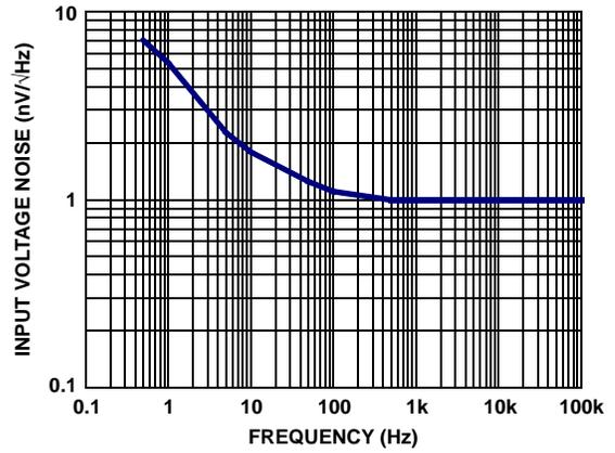
FIGURE 14. INPUT REFERRED NOISE VOLTAGE vs FREQUENCY
