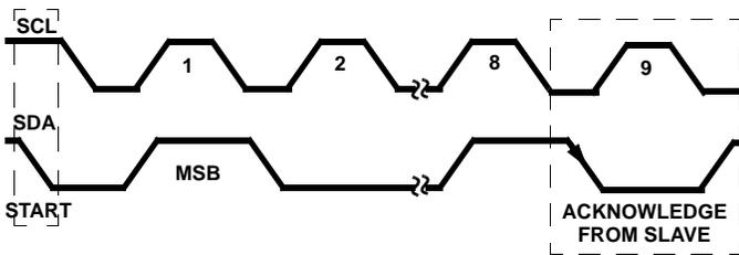
FIGURE 17. ACKNOWLEDGE ON THE I<sup>2</sup>C BUS
