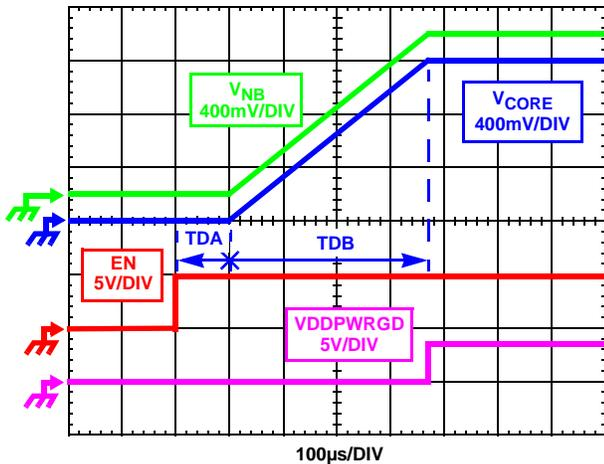
FIGURE 11. SOFT-START WAVEFORMS
