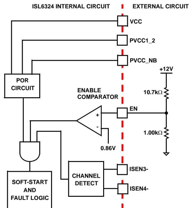
FIGURE 10. POWER SEQUENCING USING THRESHOLD-SENSITIVE ENABLE (EN)
