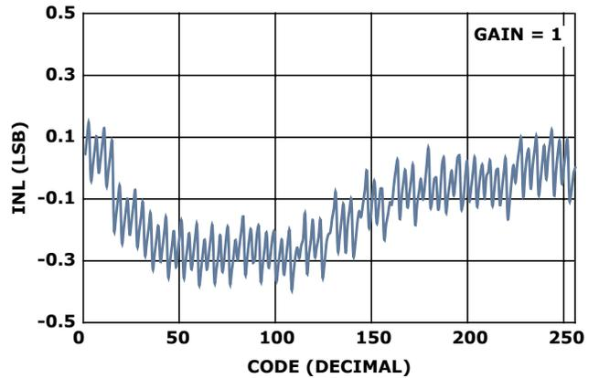
FIGURE 9. GP DAC INL vs CODE  $V_{DD} = 3V$
