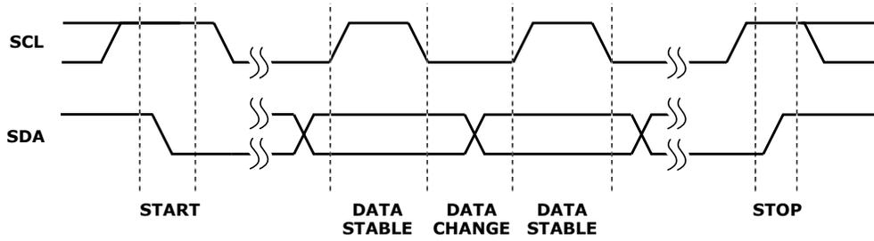
FIGURE 13. VALID DATA CHANGES, START, AND STOP CONDITIONS
