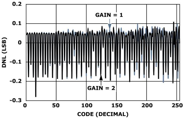
FIGURE 8. GP DAC DNL vs CODE  $V_{DD} = 15V$
