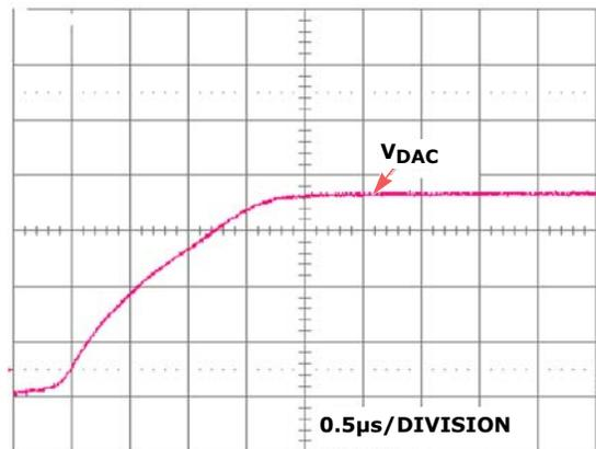
FIGURE 5. GP DAC SETTLING TIME (FULL SCALE, GAIN = 2)
