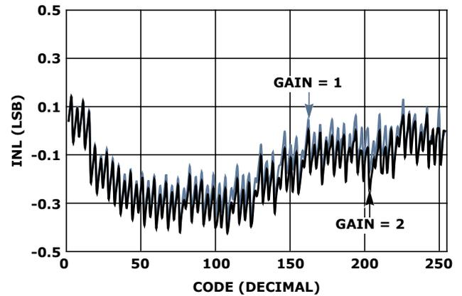
FIGURE 11. GP DAC INL vs CODE  $V_{DD} = 15V$
