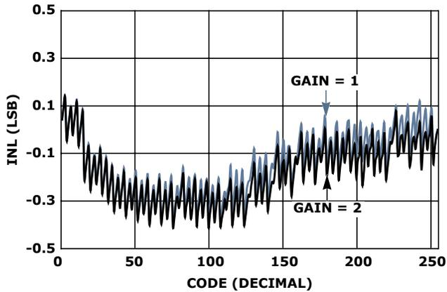
FIGURE 10. GP DAC INL vs CODE  $V_{DD} = 5V$
