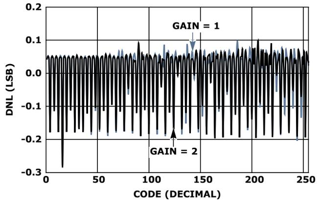
FIGURE 7. GP DAC DNL vs CODE  $V_{DD} = 5V$
