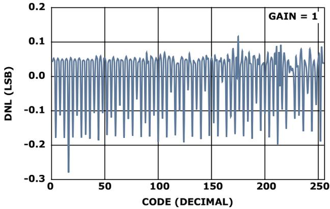
FIGURE 6. GP DAC DNL vs CODE  $V_{DD} = 3V$
