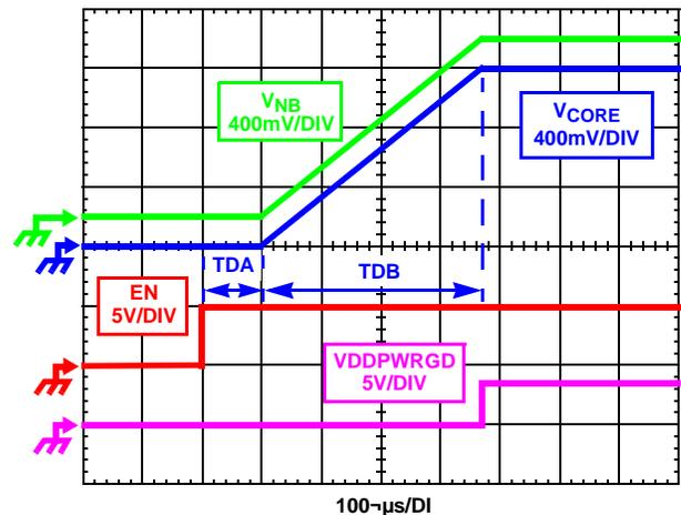
FIGURE 13. SOFT-START WAVEFORMS
