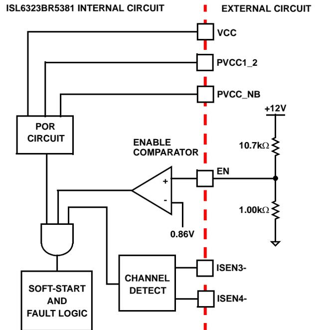
FIGURE 12. POWER SEQUENCING USING THRESHOLD-SENSITIVE ENABLE (EN)
