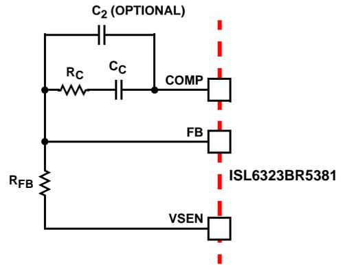
FIGURE 22. COMPENSATION CONFIGURATION FOR LOAD-LINE REGULATED ISL6323BR5381 CIRCUIT
