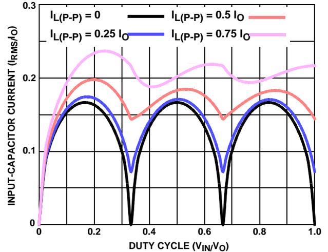
FIGURE 26. NORMALIZED INPUT-CAPACITOR RMS CURRENT FOR 3-PHASE CONVERTER
