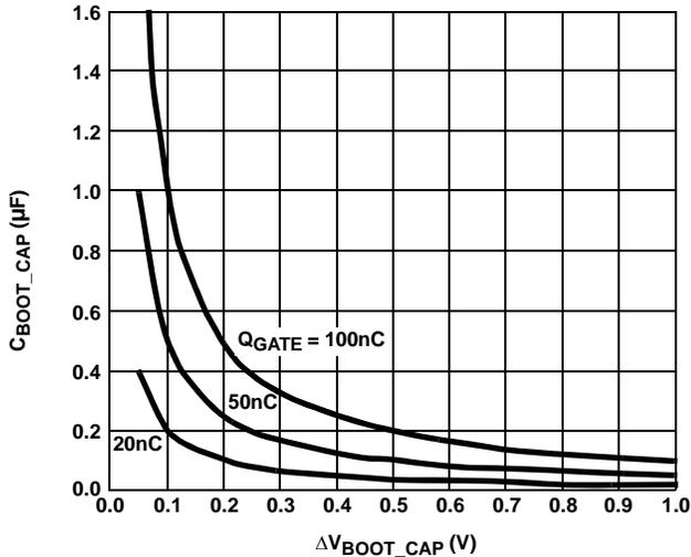
FIGURE 17. BOOTSTRAP CAPACITANCE VS BOOT RIPPLE VOLTAGE
