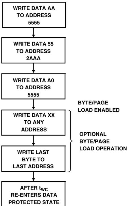
FIGURE 7. WRITE SEQUENCE FOR SOFTWARE DATA PROTECTION
