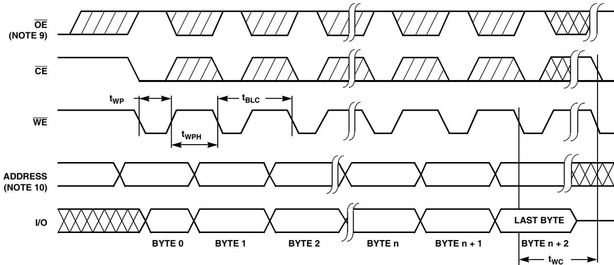
\*For each successive write within the page write operation,  $A_7$  to  $A_{15}$  should be the same or writes to an unknown address could occur.
