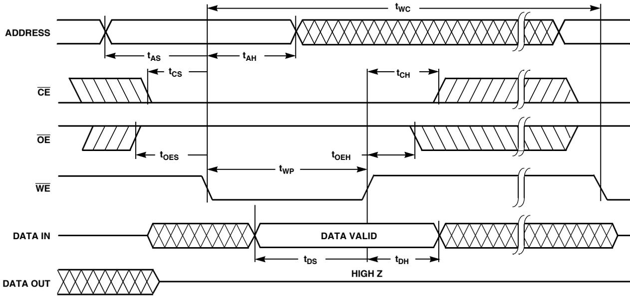
**$\overline{CE}$  Controlled Write Cycle**
