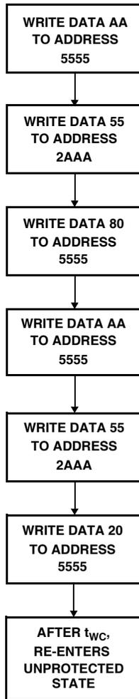
FIGURE 9. WRITE SEQUENCE FOR RESETTING SOFTWARE DATA PROTECTION
