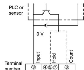
Operates when the transistor turns ON.
