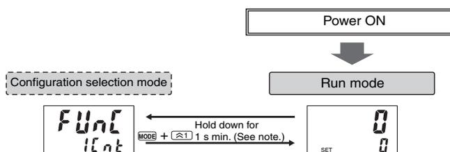
**Note:** The **MODE** key must be pressed before the **SET** key.
