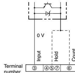
Operates when the transistor turns ON.
