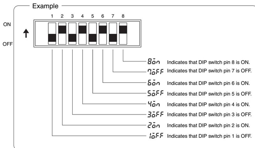
**Note:** When the mode is changed to DIP switch monitor, the measurement value is reset, outputs turns OFF, and measuring stops.
