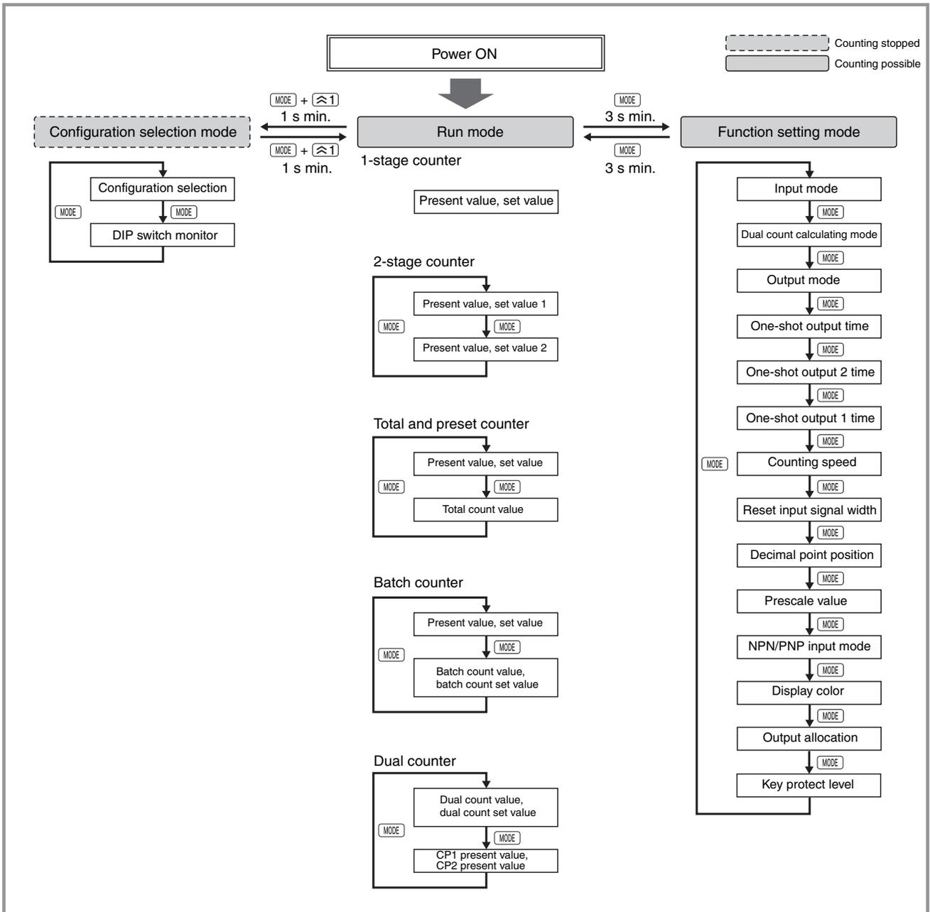
**Note:** 1. Perform settings using the  $\triangleleft$  and  $\triangleright$  keys ( $\triangleleft$  key only with 6-digit models).
