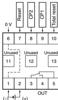
Note: Terminals 1 and 6 are connected internally.
