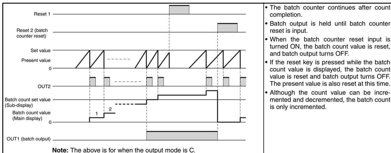
**Note:** 1. The batch count value is held at 0 during batch counter reset input.
