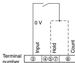
Operates when the contact turns ON.
