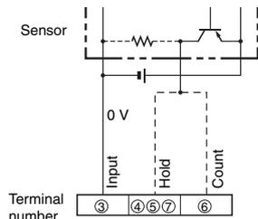
Operates when the transistor turns ON.
