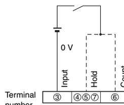
Operates when the contact turns ON.
