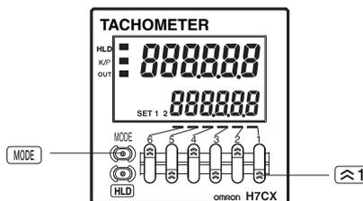
To change the mode to DIP switch monitor mode, press the MODE Key for 1 s min. with the [1] key held down. The mode will not change if the [1] key is pressed first.
