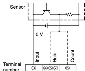
Operates when the transistor turns ON.
