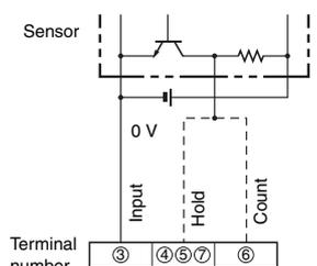
Operates when the transistor turns OFF.
