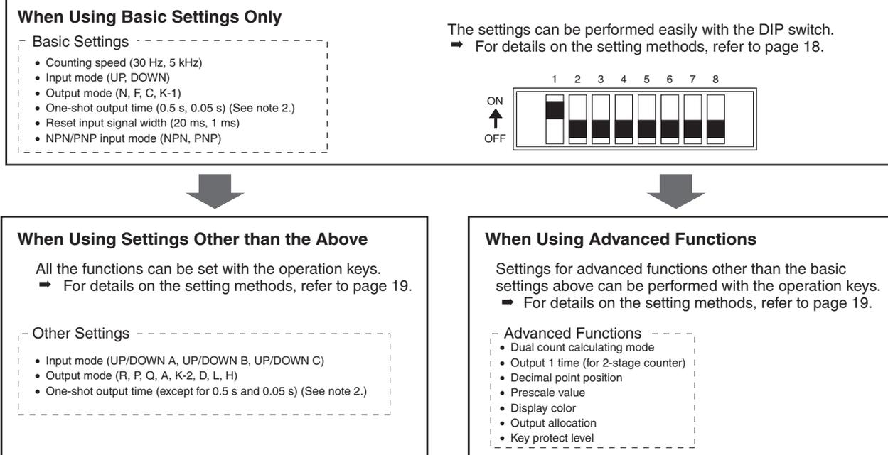
**Note:** 1. At the time of delivery, the H7CX is set to the 1-stage counter (2-stage counter for H7CX-AW□/-A4W□ models) configuration.
