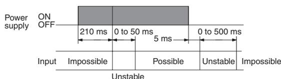
Turn the power ON and OFF using a relay with a rated capacity of 15 A minimum to prevent contact deterioration due to inrush current caused by turning the power ON and OFF.
