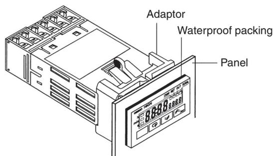
The H8GN's panel surface is water-resistant (conforming to NEMA 4X (indoors) and IP66). In order to prevent the internal circuit from water penetration through the space between the Counter and operating panel, attach a rubber packing (provided with the H8GN) between the Counter and operating panel and secure the rubber packing with the Flush-mounting Adaptor.
